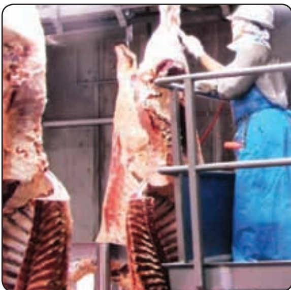
RFP allows the worker to maintain the optimal working position to the carcass.
