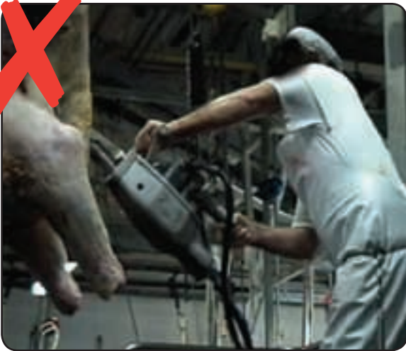
Reaching and poor posture should be kept to a minimum. (See next page for photo of optimum manual handling practice for this task.)
